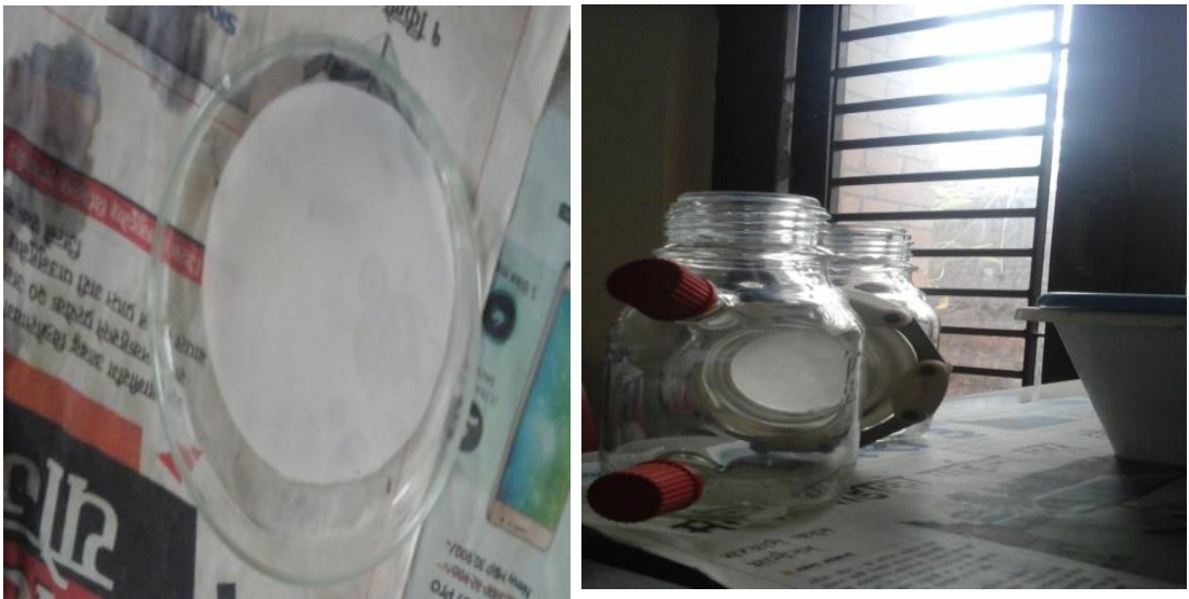
Figure A8: Left: Membrane coated with cellulose acetate. Right: Electrochemical Cell with cellulose acetate coated membrane.
