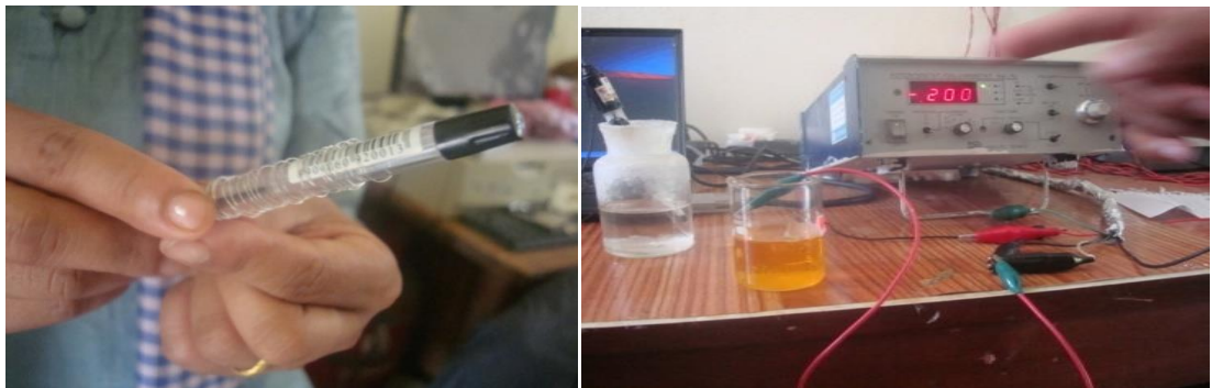
Figure A5: Left: Platinum wire.. Right: Electroplating of platinum wire
