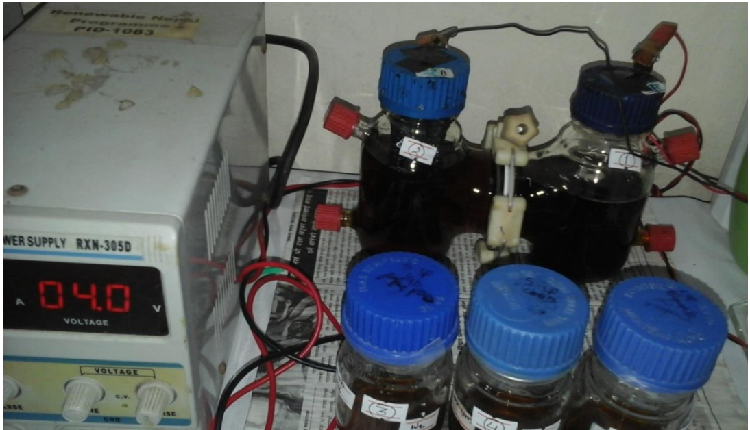
Figure A7: Electrochemical cell with S. spontaneum hydrolysate as media along with normal fermentation of cultures.
