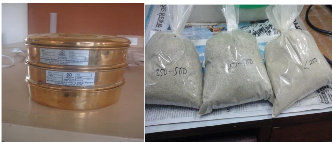
Figure A3: Photographs Left: Sieve for obtaining required particle size of biomass, Right: Biomass with different particle size stored in plastic pouch.
