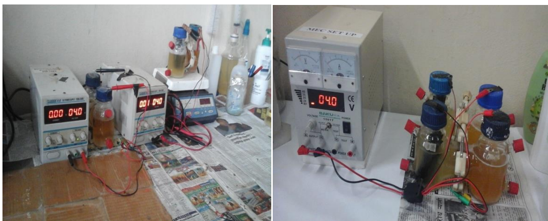
Figure A6: Electrochemical cell (PYN media supplied with glucose and with voltage supply).
