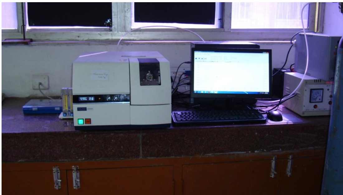
Figure A11: Thermo gravimetric analyzer (TGA) (STA 7200 HITACHI) attached with PC available in Biotechnology Lab, IITG, Guwahati.
