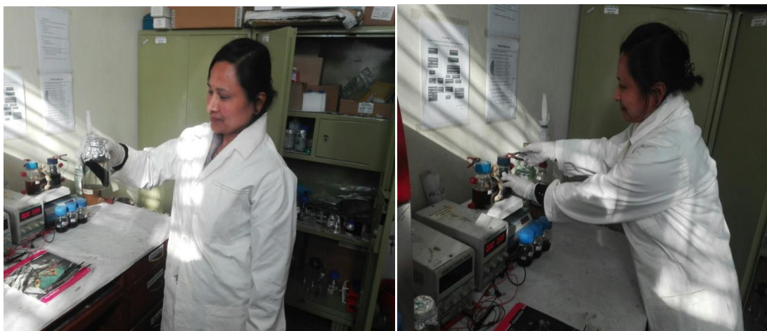
Figure A13: Photographs Left: Cleaning graphite electrode. Right: Installing ECC.
