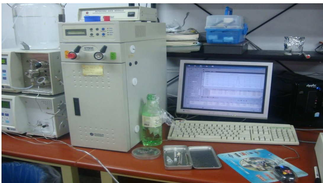
Figure A12: HPLC analyzer (Agilent with RI detector) attached with PC available in Department of Chemistry IITG, India.
