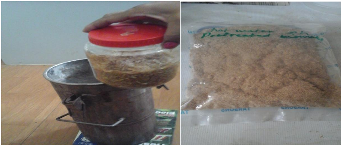
Figure A4: Photographs Left: Biomass keeping in pretreatment vessel for pretreatment. Right: Biomass stored in plastic pouch after pretreatment and drying.
