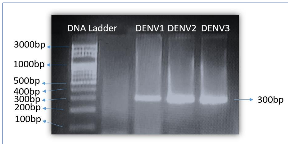
Fig 4. 5. Gel images under UV Transilluminator of the second round nested PCR of envelope Domain III region that 299 bp amplicon corresponds to DENV1, 306 bp amplicon corresponds to DENV2 and 296 bp amplicon corresponds to size of DENV3. 100bp DNA ladder was used to determine size around 300bp representing all serotypes.
