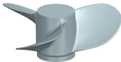
Figure 3.3 Final CAD Geometry
