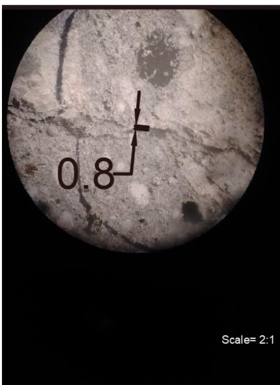
Images 12,13,14,15: Optical images of cracks after 10 days
