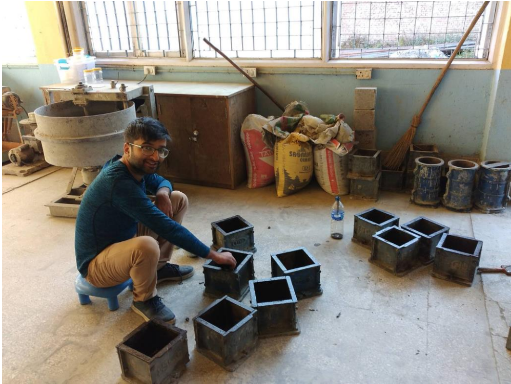
Image 32: Cube molds preparation
