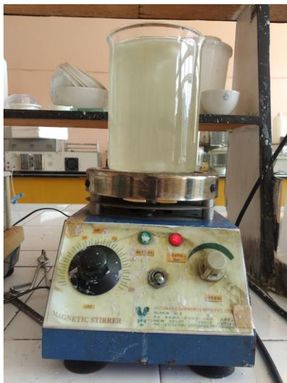
Image 24: Precursor Solution preparation on magnetic stirrer
