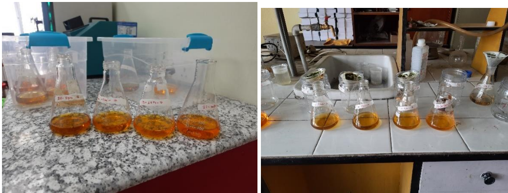
Figure B10: Decolorizations of MO dye after exposing azolla for 7 days
