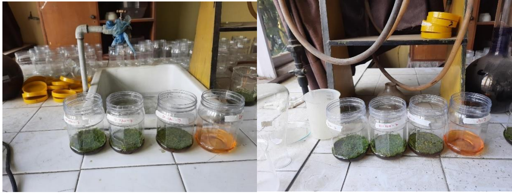
Figure B8: Layout of Phytoremediation of MO dye by Azolla Pinnata
