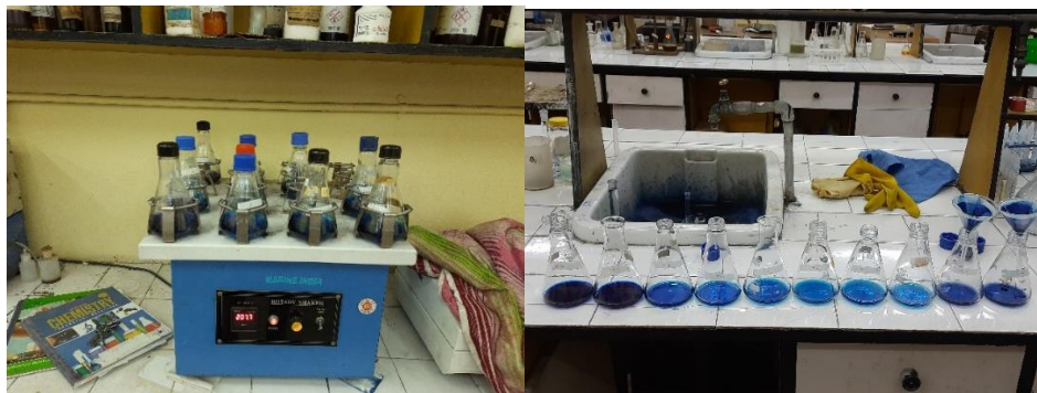
Figure B10: Decolorizations of MO dye after exposing azolla for 7 days
