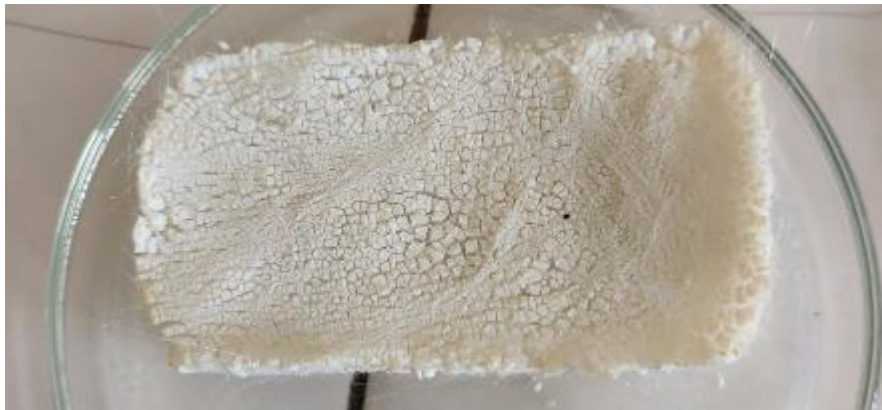
Figure 4.37: Presence of cracks
