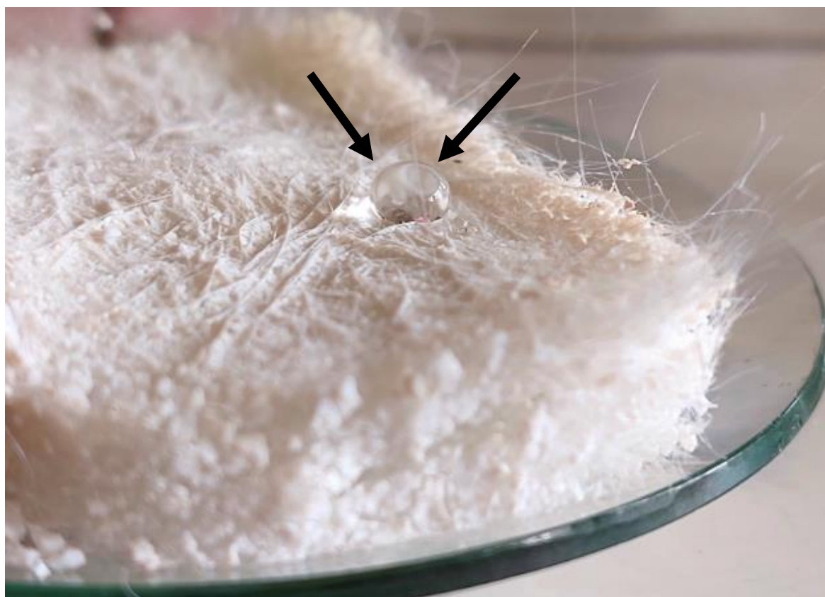
Figure 4.36: Visual inspection of WW2 for hydrophobicity after heating at 200°C
