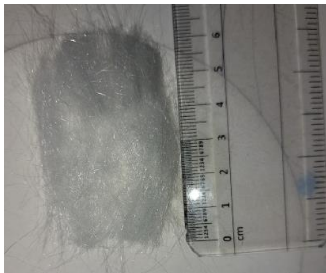
Figure 3.2: Glass wool used for reinforcement
