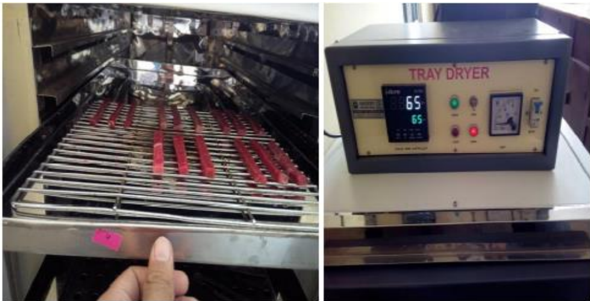
Plate 2 Drying of jerky after marination with humectants mixture
