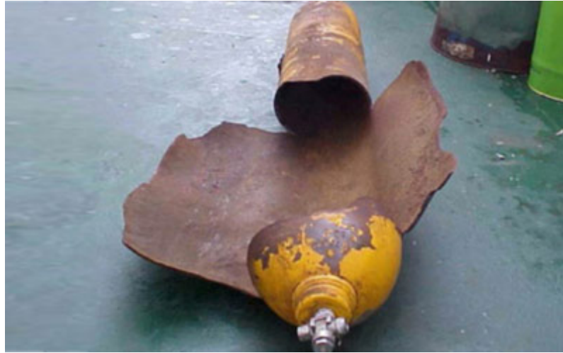
Figure 1.2: Bursted Oxygen Cylinder (source:safetymattersweekly.com)
