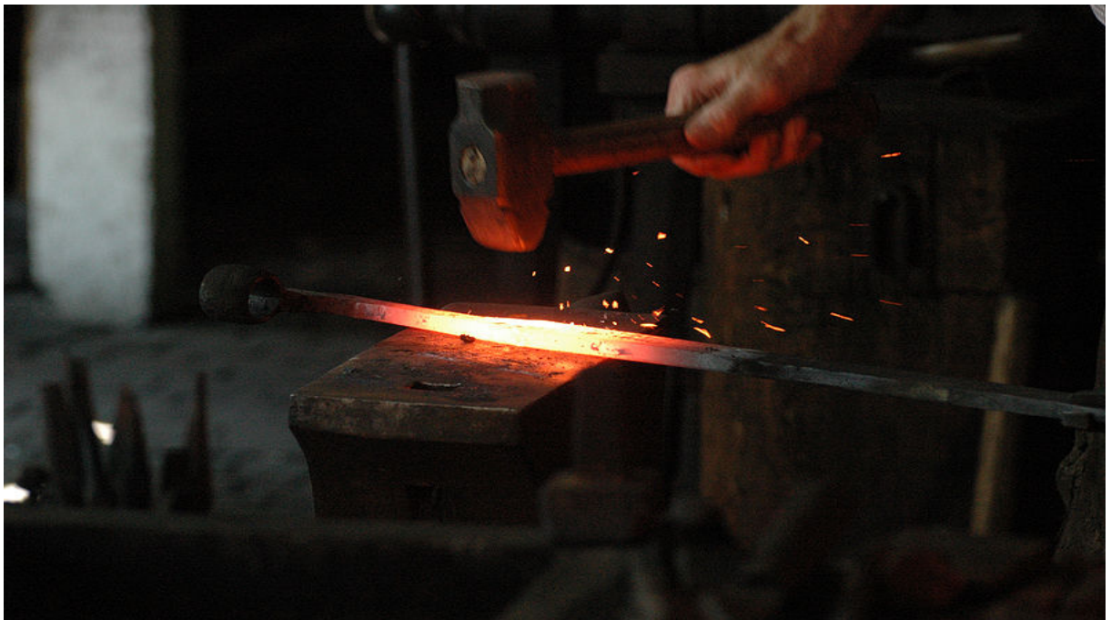
Figure 1.3: Blacksmith working on hot iron [2].
