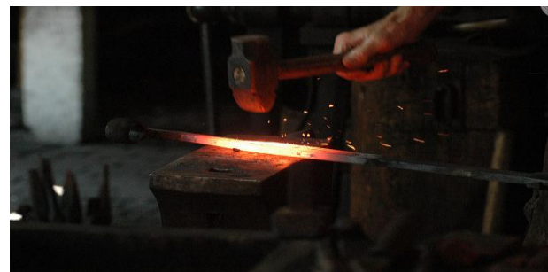
Fig. 2: Blacksmith working on hot iron [23].
