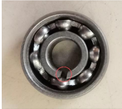
Figure 4. 3: Inner Raceway Fault
