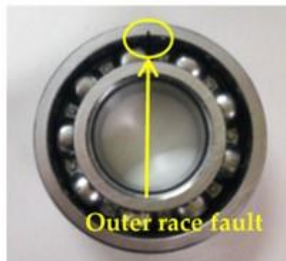
Figure 1. 3: Outer Raceway Fault
