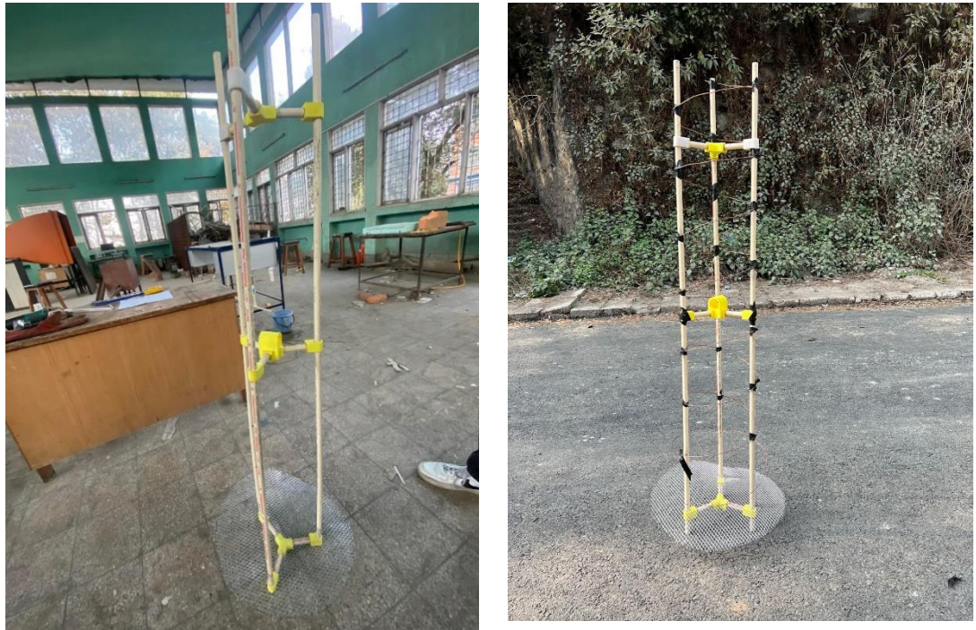
Figure 5.5: Making of Helical Antenna (left) and Completed Helical Antenna (right)
