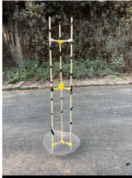
Figure C.1: Construction of Antenna
