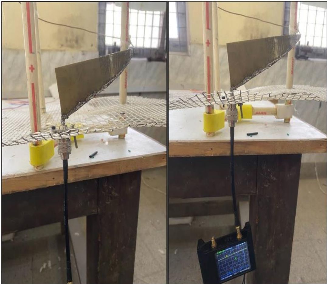
Figure 5.6: Brass Plate, wire and N -type connector being soldered (Left) Impedance Matching Being Checked (Right)
