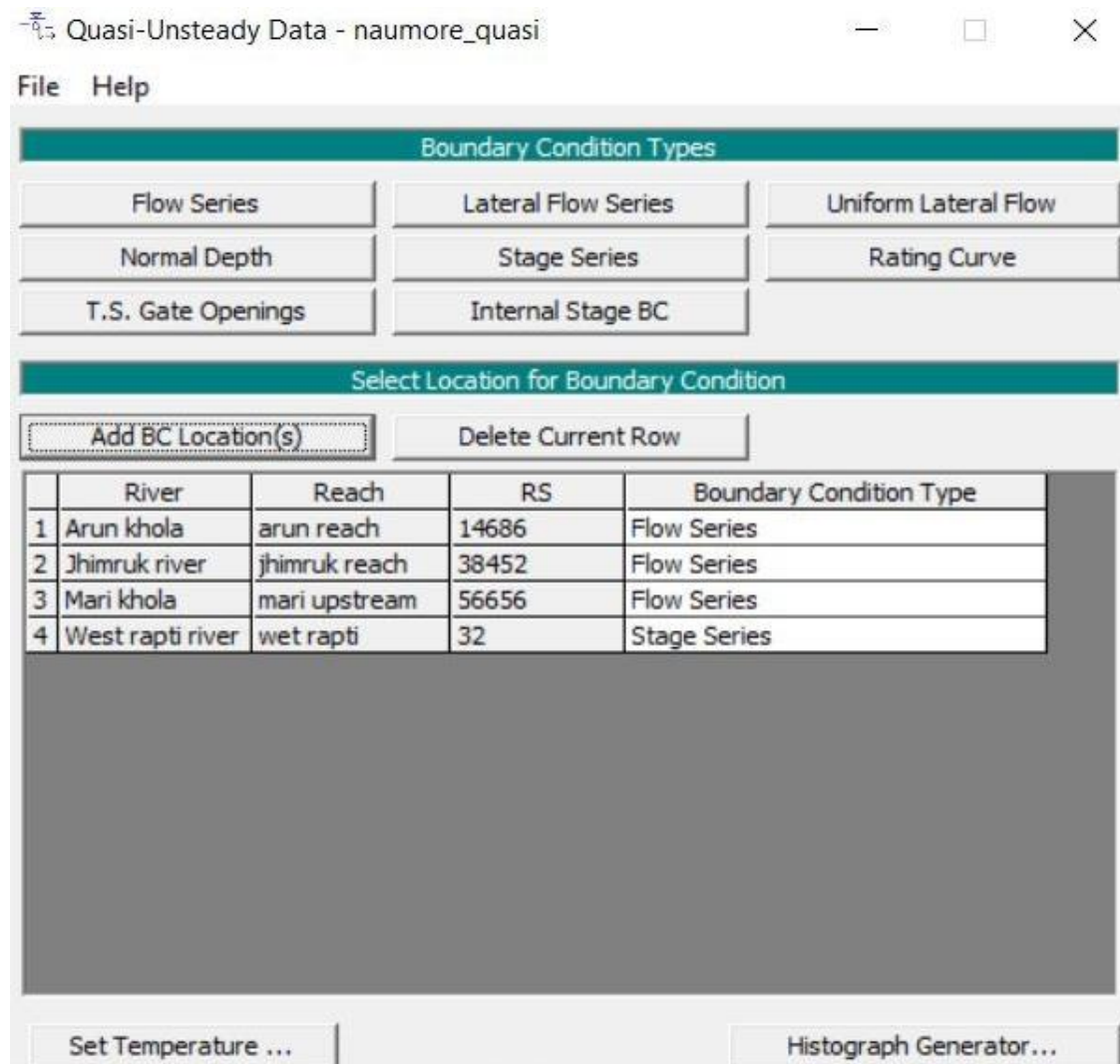
Figure 4-3 Flow Boundary Condition
