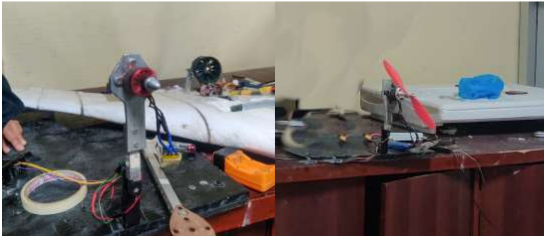
Fig 4. 31: Measurement of thrust using thrust stand
