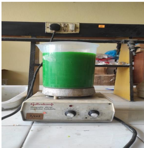
Figure 19 Synthesis of nanofluid using magnetic stirrer
