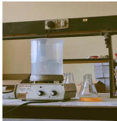
Figure 19 Synthesis of nanofluid using magnetic stirrer
