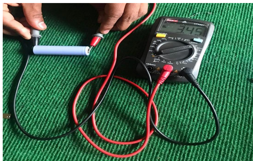
Figure 3-3: Open circuit voltage measurement
