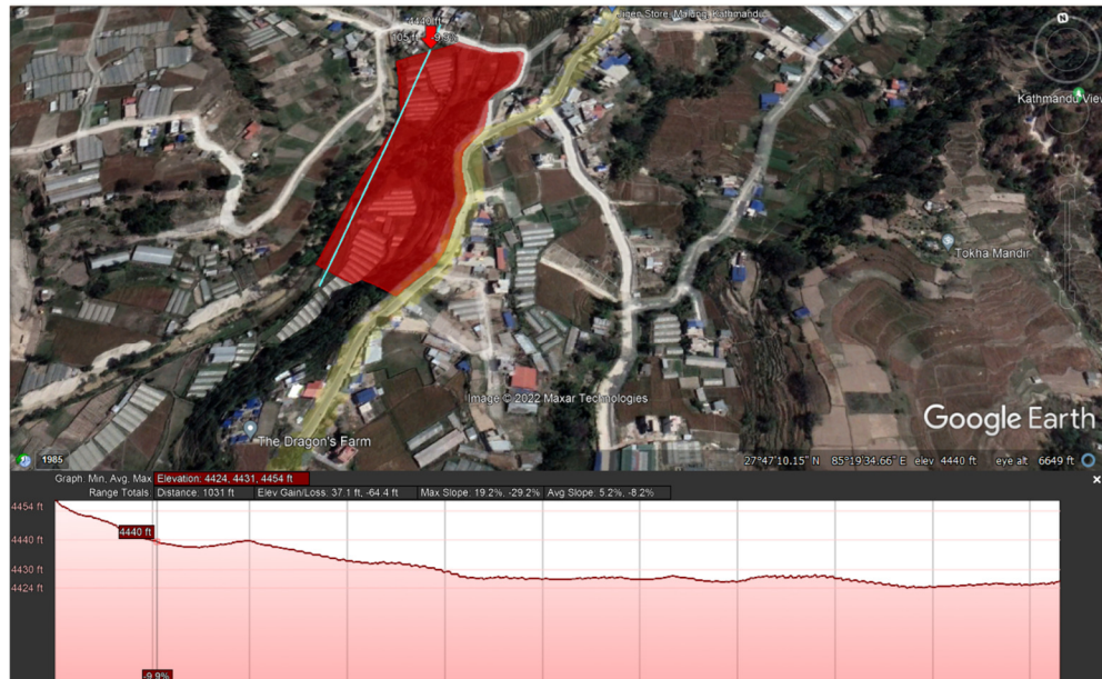
Figure 39 longitudinal section of the site
