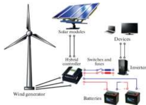
Figure 14: wind solar hybrid power system
