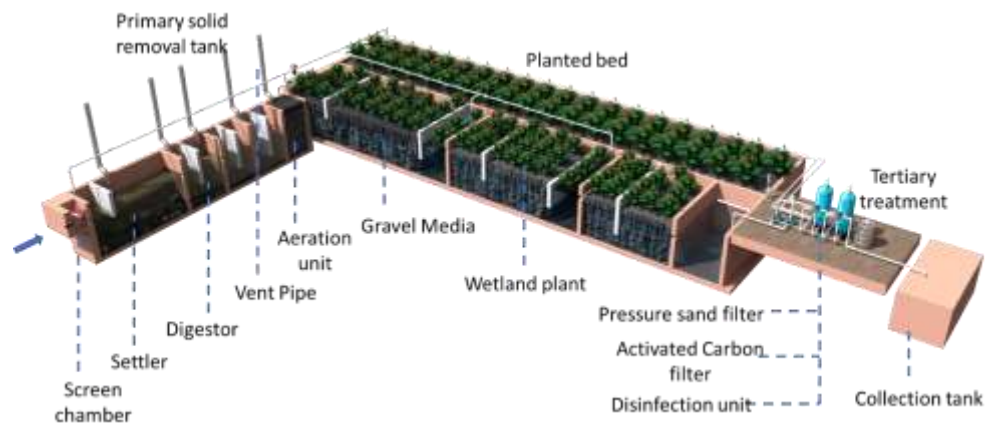
Figure 57: Natural grey water treatment
