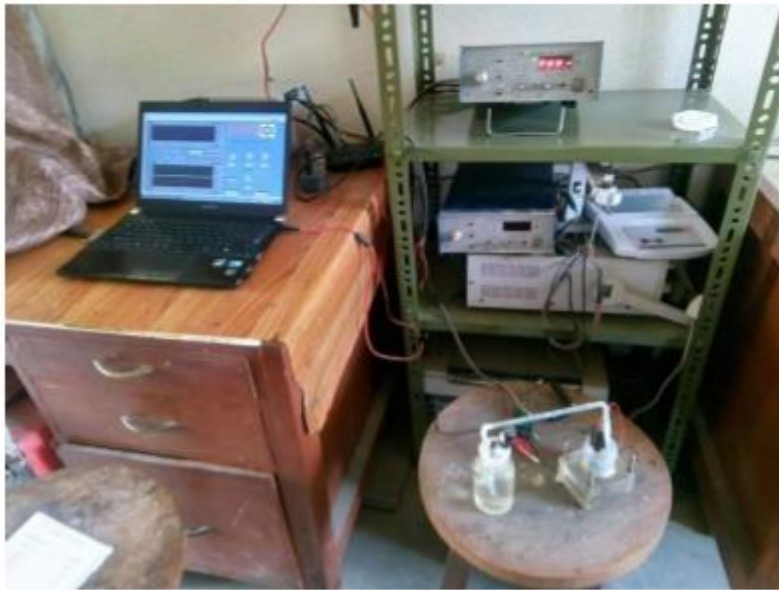
Figure 3.2: Experimental set up for potentiodynamic polarization of mild steel
