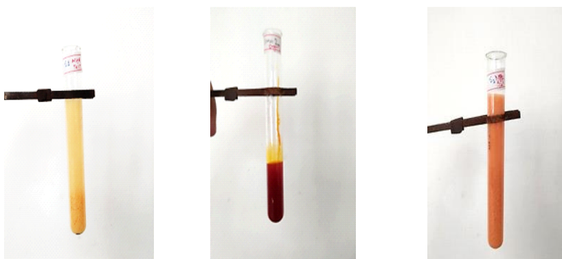
Figure 4.1: Test for alkaloids: a) Mayer's b) Dragendroff's and c) Wagner's test
