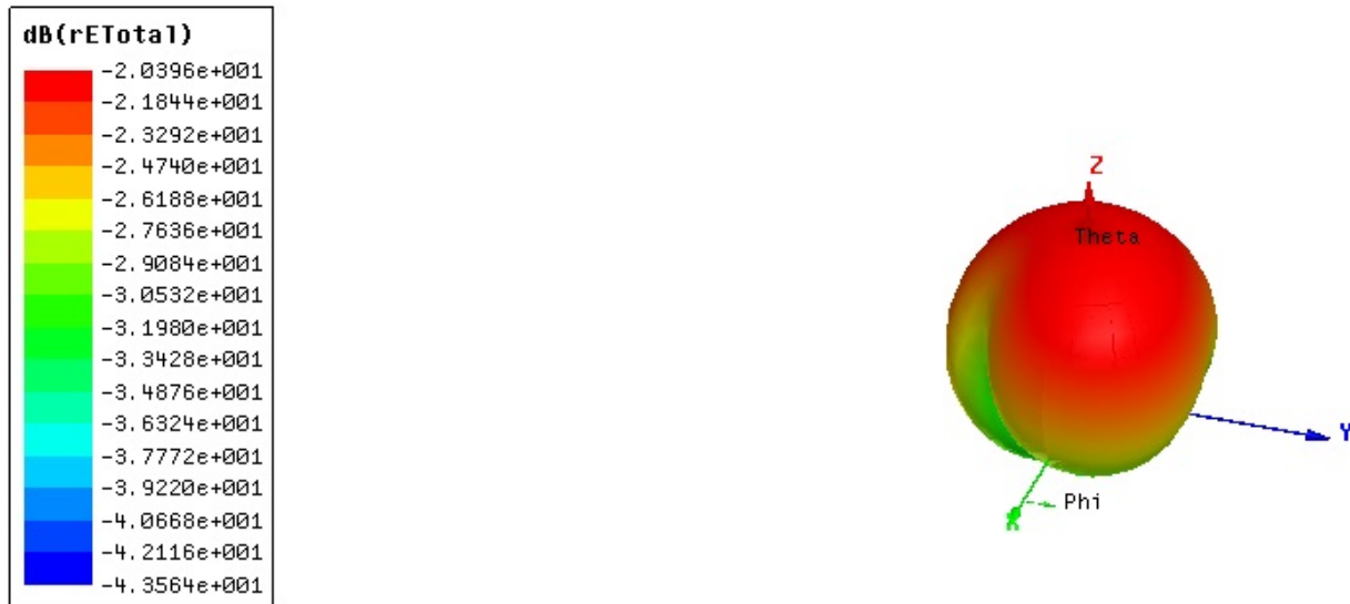
Figure 5.34: 3-D polar plot gain of swastika slot antenna of graphite as patch and copper as ground in polycarbonate substrate
