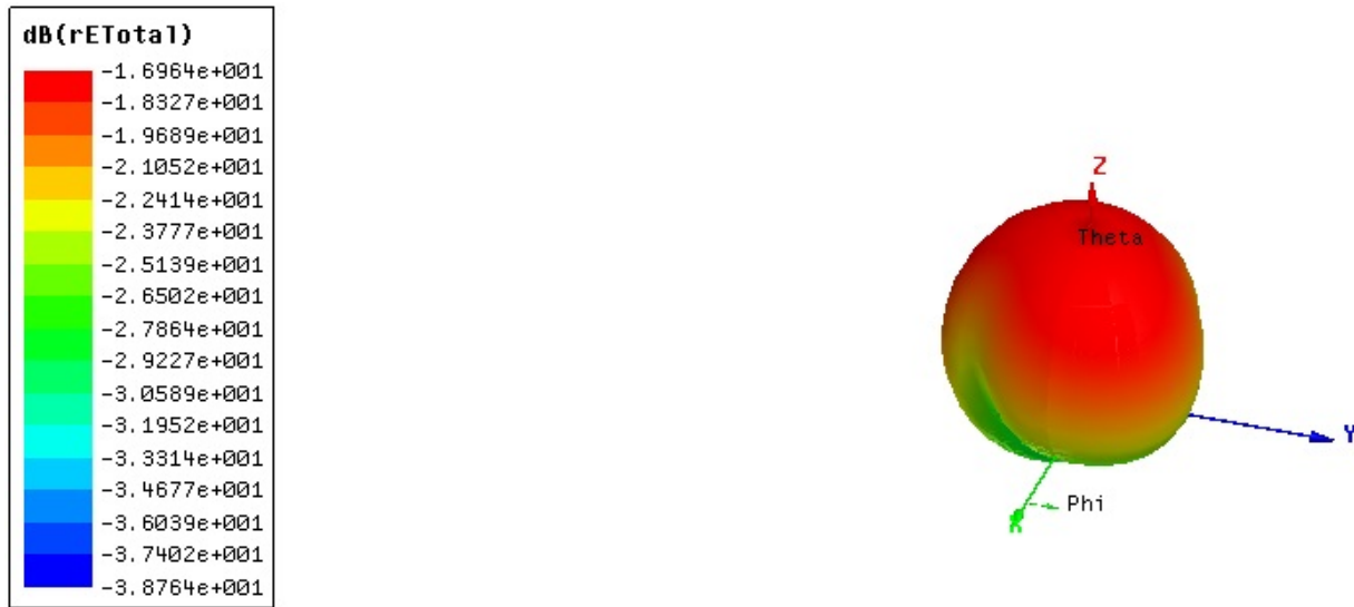
Figure 5.29: 3-D polar plot gain of swastika slot antenna of copper as patch and copper as ground in polycarbonate substrate
