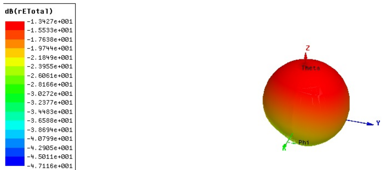
Figure 5.39: 3-D polar plot gain of swastika slot antenna of copper as patch and copper as ground in corning glass substrate
