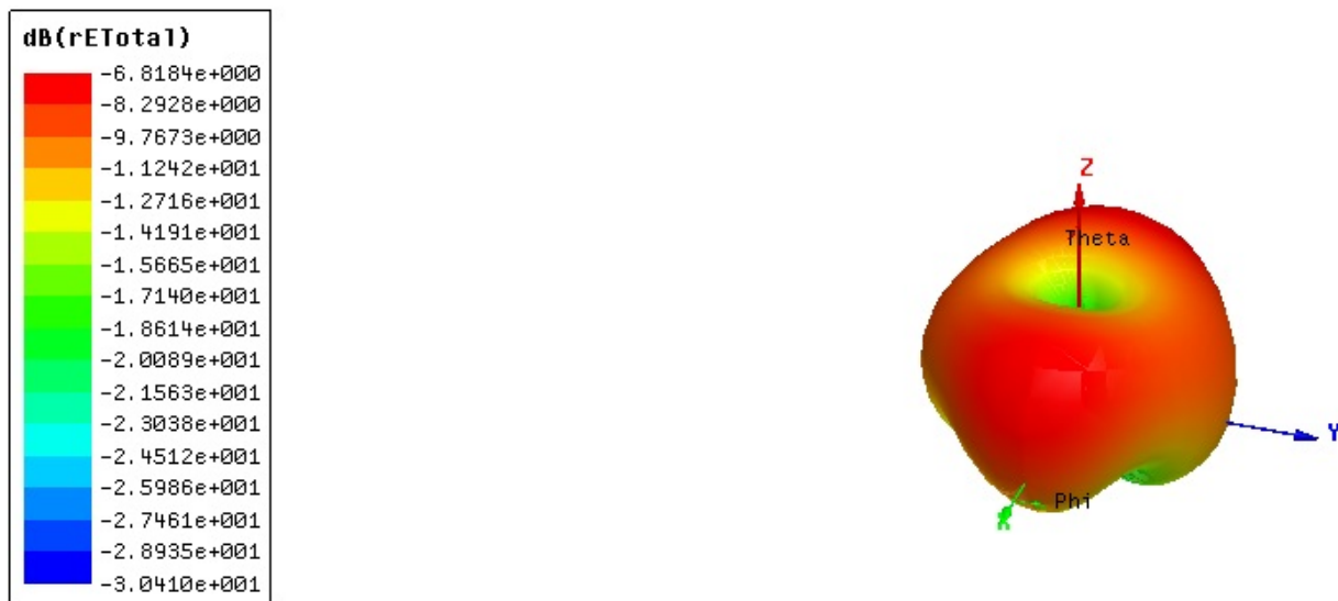
Figure 5.19: 3-D polar plot gain of reference antenna of copper as patch and copper as ground in corning glass substrate
