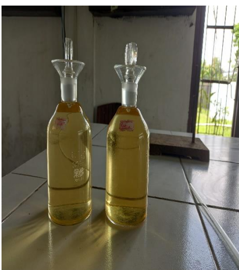
Photo 32: Water samples for titration of DO
