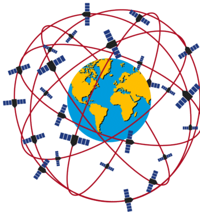
Figure 26: Six different orbital planes of GPS system ( https://seos-project.eu/GPS/GPS-c01-p03.html ).
