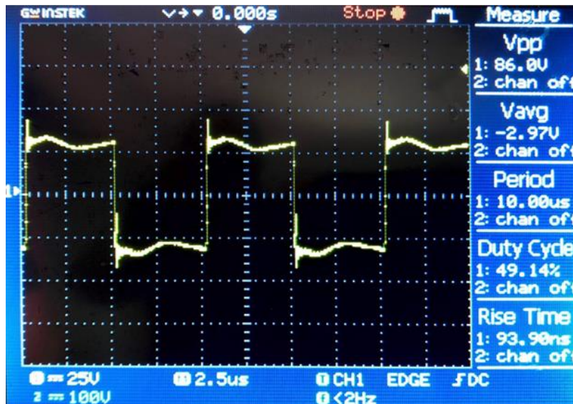
Figure 4. 27: The Output of the Inverter
