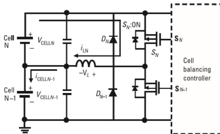
FIGURE3. 1 BALANCING CIRCUIT DIAGRAM [10]
