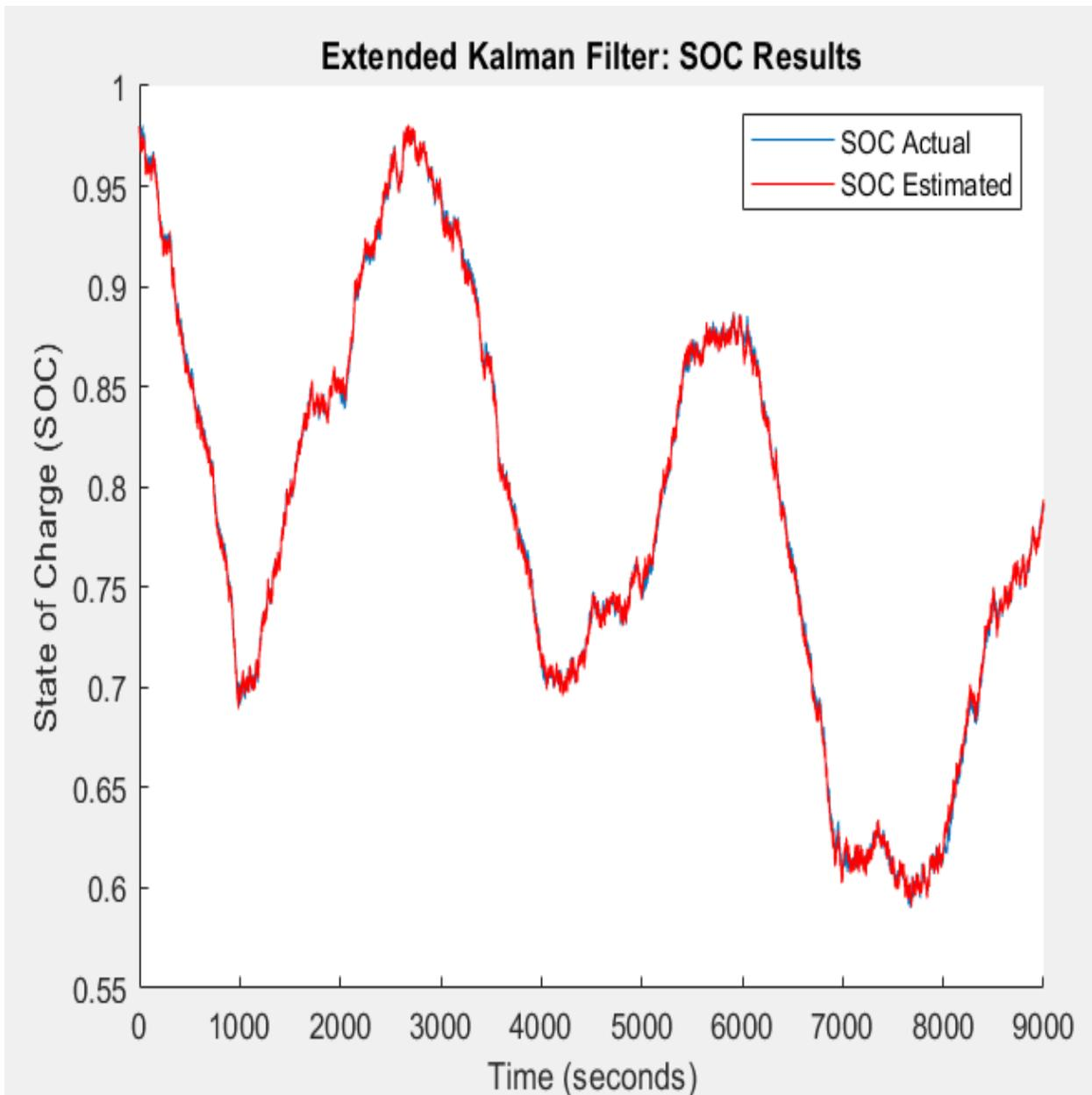
**FIGURE 4. 4 ACTUAL SOC AND ESTIMATED SOC VS TIME**
