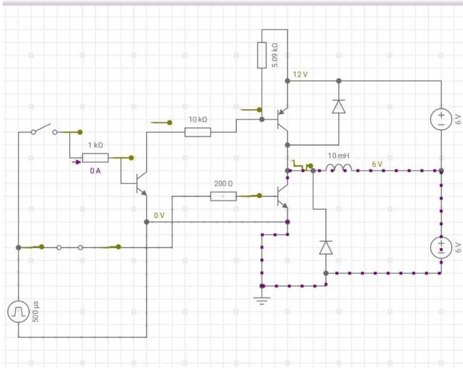
**FIGURE 4. 9 BALANCING CIRCUIT DIAGRAM WHEN SOC OF LOWER CELL IS GREATER THAN LOWER CELL**
