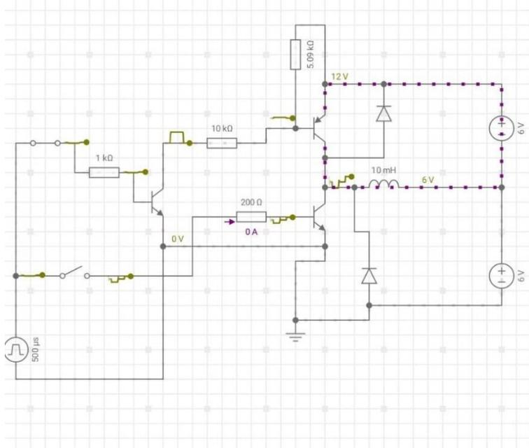
FIGURE 4. 7 BALANCING CIRCUIT DIAGRAM WHEN SOC OF UPPER CELL > THAN LOWER CELL
