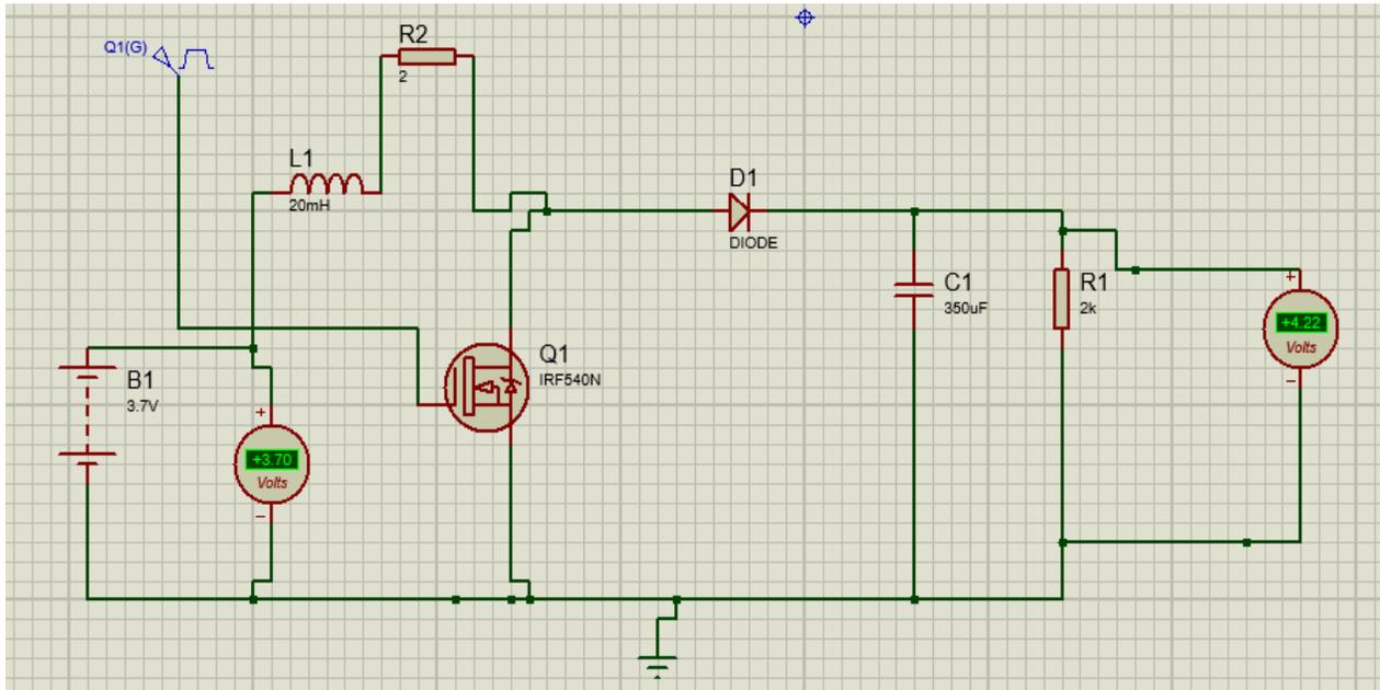
FIGURE 4. 14 BOOST CONVERTER CIRCUIT IN PROTEUS
