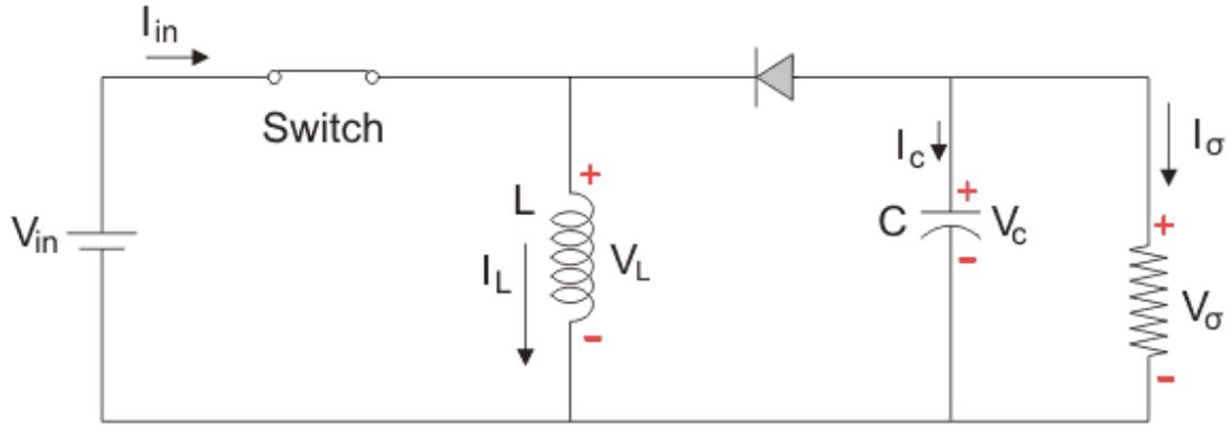
**FIGURE 2. 3 OPERATION OF BUCK BOOST CONVERTER WHEN SWITCH IS ON [8]**
