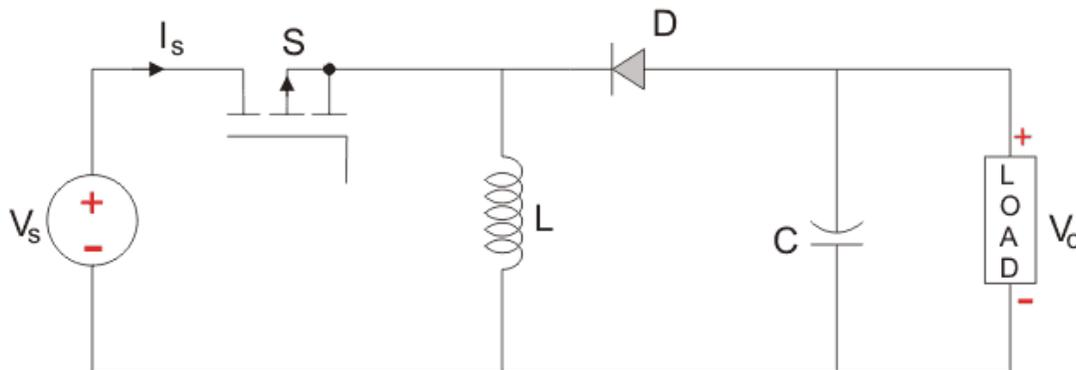
**FIGURE 2. 2 BUCK BOOST CONVERTER [8]**
