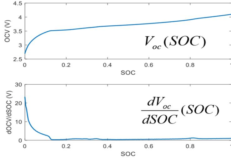
**FIGURE 4. 1 OCV VS  $V_{oc}$  AND  $\frac{dOCV}{dSOC}$  vs SOC**
