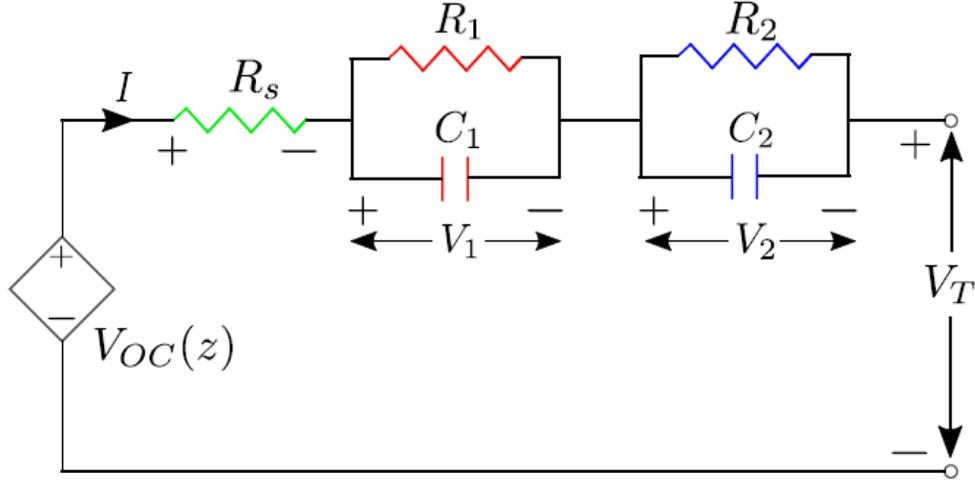
FIGURE 2. 5 DUAL POLARITY MODEL [9]
