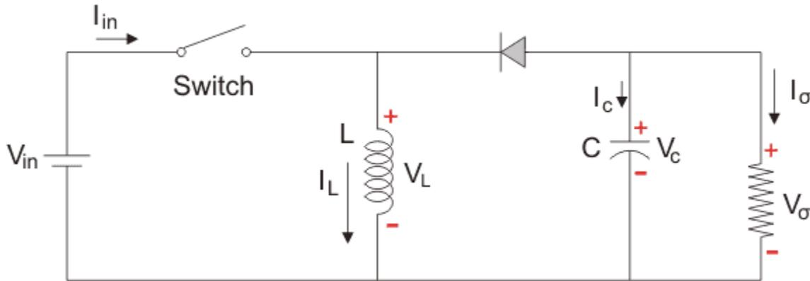
**FIGURE 2. 4 OPERATION OF BUCK BOOST CONVERTER WHEN SWITCH IS OFF [8]**
