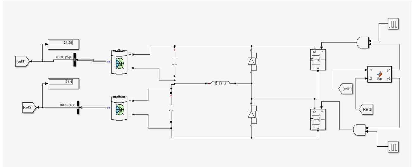
**FIGURE 4.5 SIMULATION OF ACTIVE CELL BALANCING CIRCUIT IN MATLAB**
