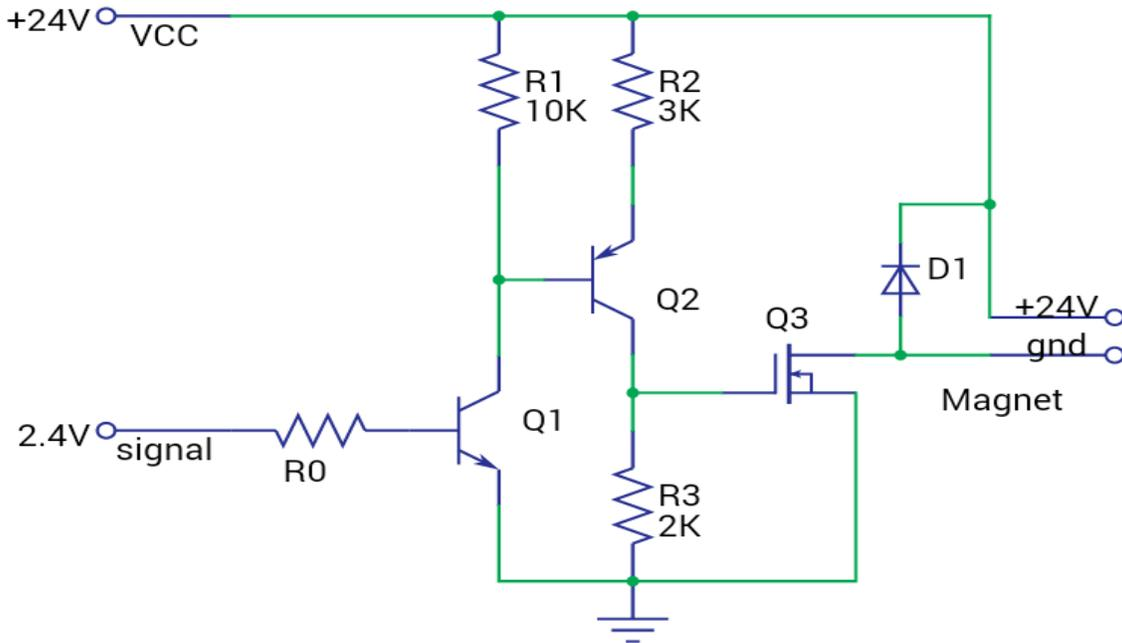
FIGURE 4. 11 MOSFET DRIVING CIRCUIT
