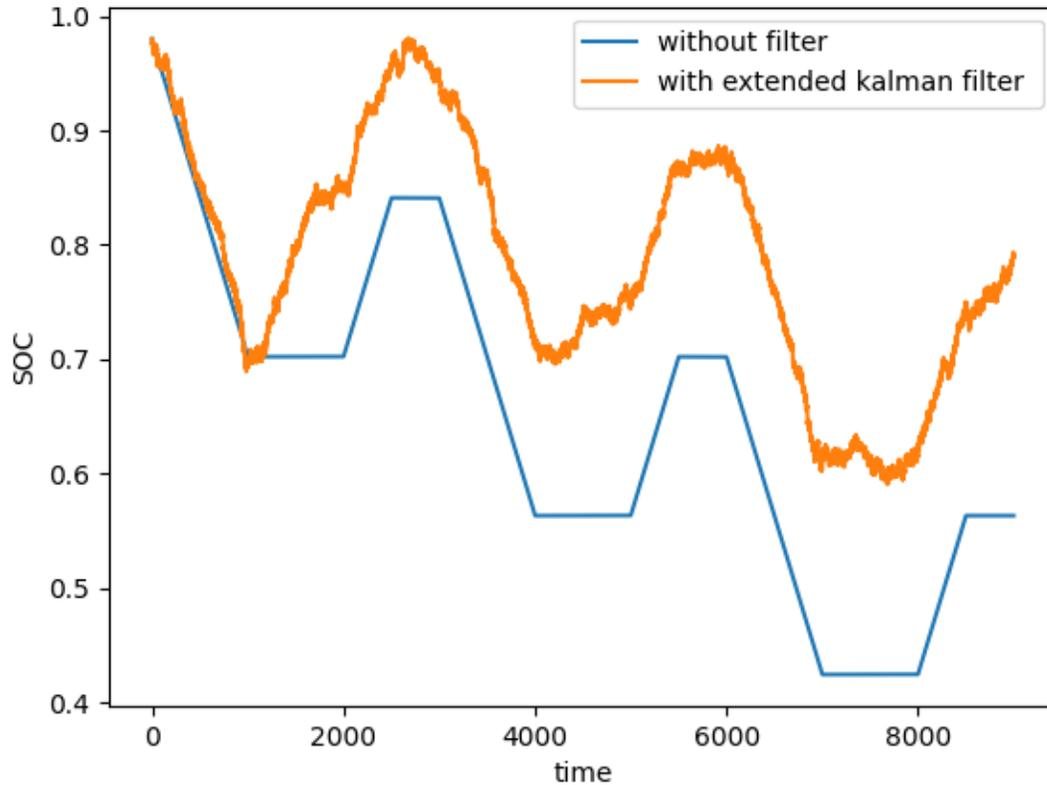
**FIGURE 4.6 SOC VS TIME WITH AND WITHOUT EXTENDED KALMAN FILTER**
