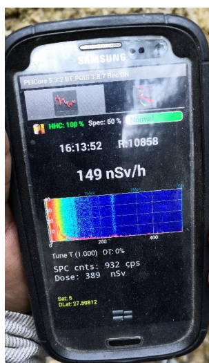
Figure 9: Instant spectrum and dose rate displayed on mobile screen during survey
