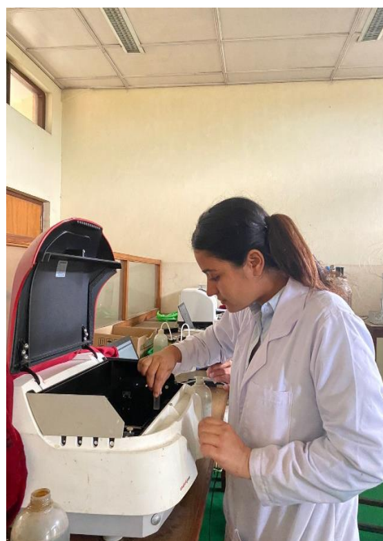
Taking the absorbance in UV-Visible spectrophotometer
