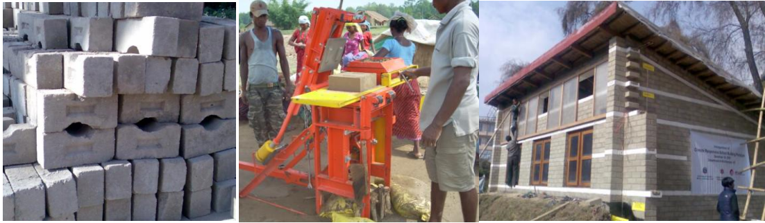
Fig. 6.13 Views of CSEB block, manufacture of CSEB by AURAM -300 machine and the CSEB model classroom building in the Department of Architecture, Pulchowk campus, Lalitpur, Nepal
