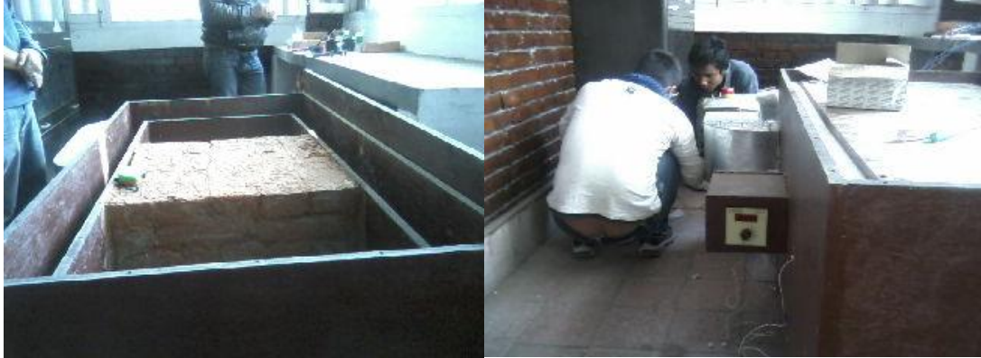
Fig. 6.2 A wall constructed for experiment in the insulated thermal box in the laboratory
