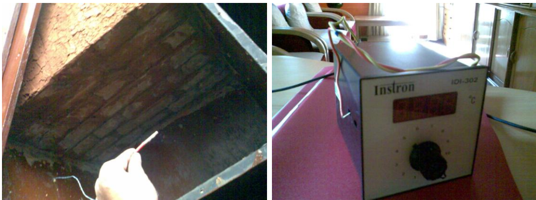
Fig. 3.4 Views of sensor R6, wall inside the thermal box and multiple temperature recorder (Instron IDI-302) in a lab for Mini research
