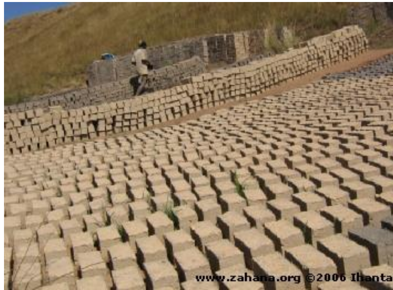
Fig. 6.3 View of manufacture of Sun dried brick ( Kachi Apa ) in Kathmandu valley
