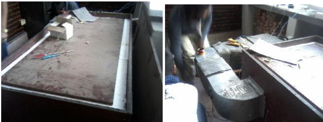
Fig. 6.1 An insulated thermal box with air conditioning system in a building science laboratory, Department of Architecture, Pulchowk Campus
