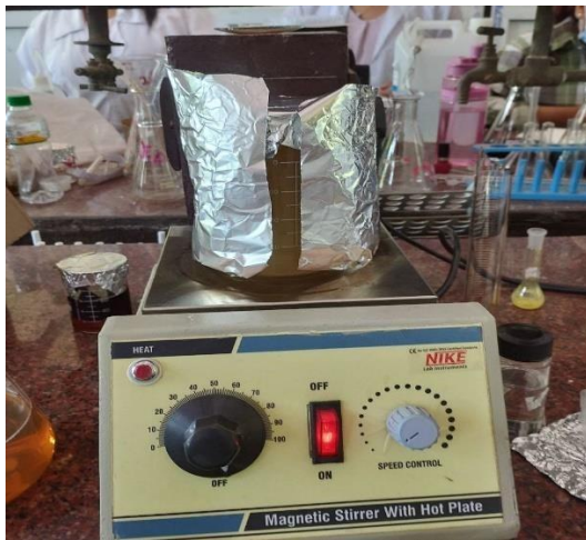
Plant extract + silver nitrate in magnetic stirrer
