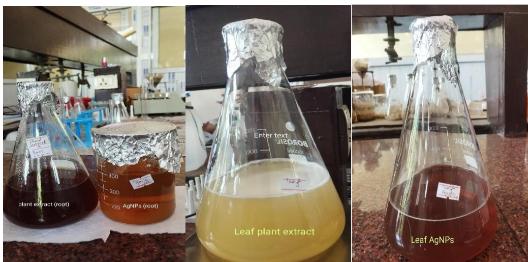
Figure 26: Visible observation of color change of plant extract after the addition of silver nitrate
