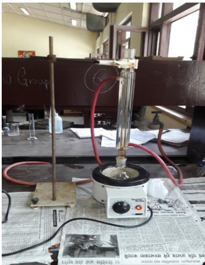
Fig. 4.2 (a) Oxidation of Multi-walled carbon nanotubes through acid reflux Process
