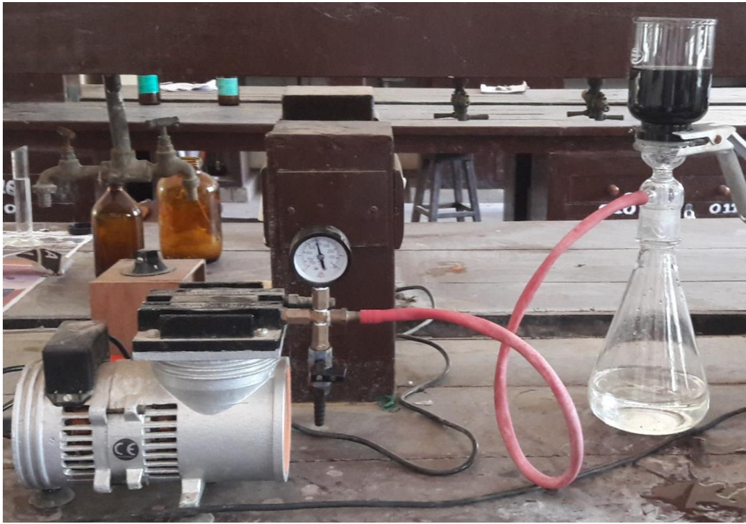
Fig 4.2 (c) Purification of oxidized Multi-walled carbon nanotubes using Suction pump
