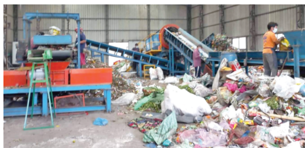
Figure 24: Waste segregation and processing, Source: Venture WTE, Pvt. Ltd.
