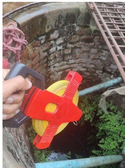
Figure 38:- Measurement of water level of well
