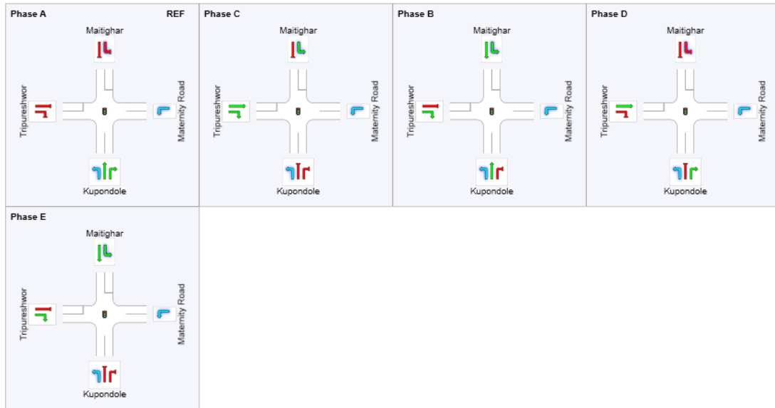
Figure 4-39: Phase plan for the weekday model with geometric enhancements
