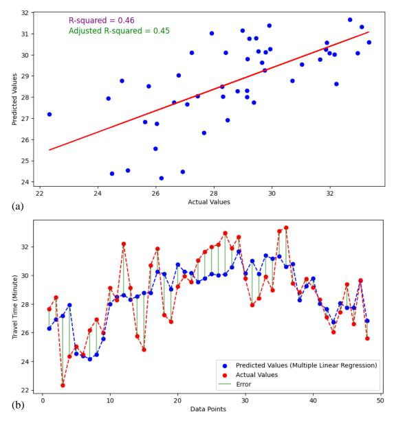
Figure 5-3: Travel Time Prediction based on Multiple Linear Regression model for Bhaluwang to Dhankhola direction (a) Prediction (b) Distribution of tested and predicted error
