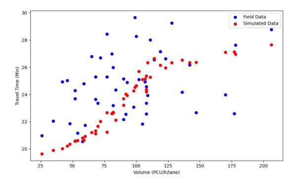
Figure 6-2: Comparison of Travel Time-Volume Relationship from field dCoata and simulation result
