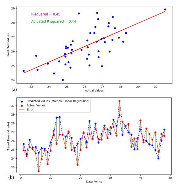
Figure 5-2: Travel Time Prediction based on Multiple Linear Regression model for Dhankhola to Bhaluwang direction (a) Prediction (b) Distribution of tested and predicted error
