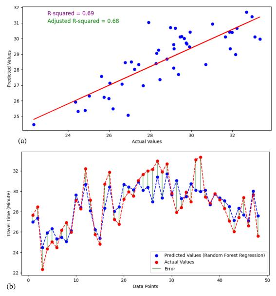
Figure 5-11: Travel Time Prediction based on Random Forest Regression model for Bhaluwang to Dhankhola direction (a) Prediction (b) Distribution of tested and predicted error
