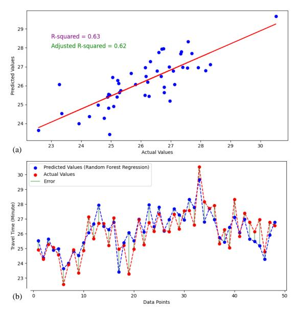
Figure 5-10: Travel Time Prediction based on Random Forest Regression model for Dhankhola to Bhaluwang direction (a) Prediction (b) Distribution of tested and predicted error
