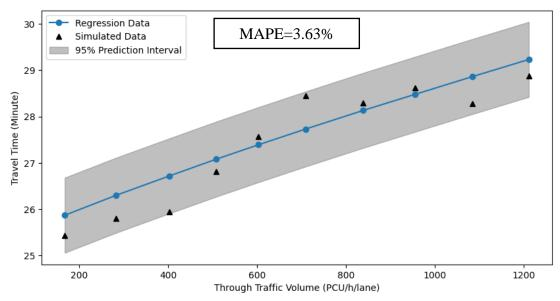
Figure 6-7: Validation of proposed travel time function of heavy vehicles- case I
