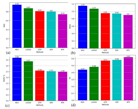
Figure 5-12: Comparison of regression results and statistical errors of prediction models at Dhankhola to Bhaluwang direction: (a) MAE (b) RMSE (c) MAPE (d) R<sup>2</sup>
