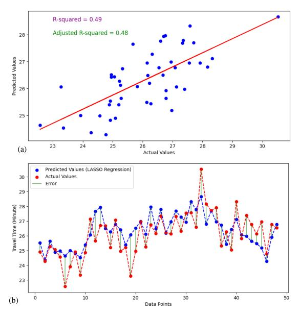
Figure 5-4: Travel Time Prediction based on LASSO Regression model for Dhankhola to Bhaluwang direction (a) Prediction (b) Distribution of tested and predicted error
