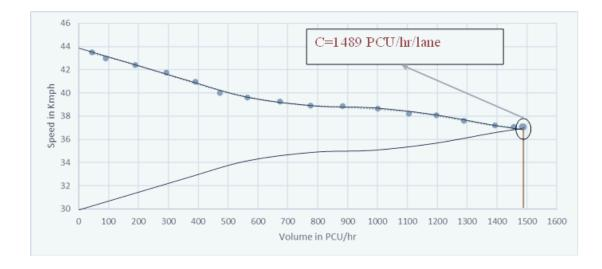
Figure 6-4: Relationship between speed and flow
