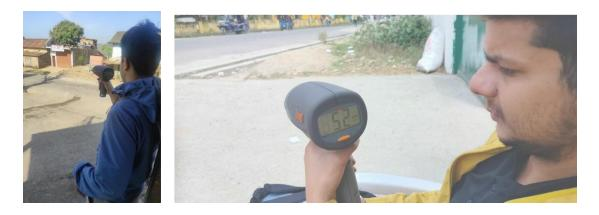
Figure 3-6: Spot speed survey using radar gun
