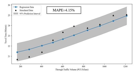
Figure 6-6: Validation of proposed travel time function of light vehicles
