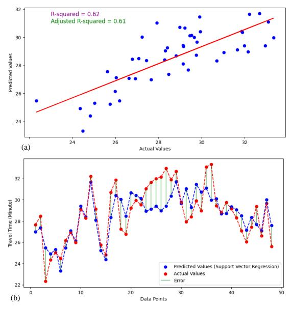
Figure 5-9: Travel Time Prediction based on Support Vector Regression model for Bhaluwang to Dhankhola direction (a) Prediction (b) Distribution of tested and predicted error
