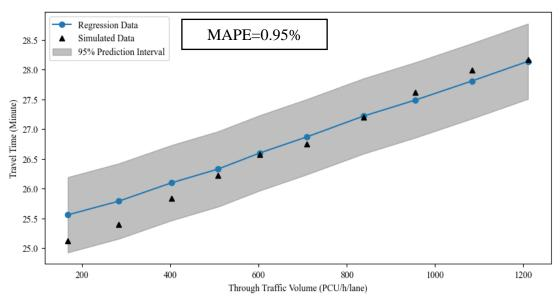
Figure 6-8: Validation of proposed travel time function of heavy vehicles- case II
