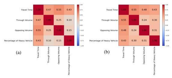
Figure 5-1: Correlation Matrix: (a) Dhankhola to Bhaluwang direction (b) Bhaluwang to Dhankhola direction
