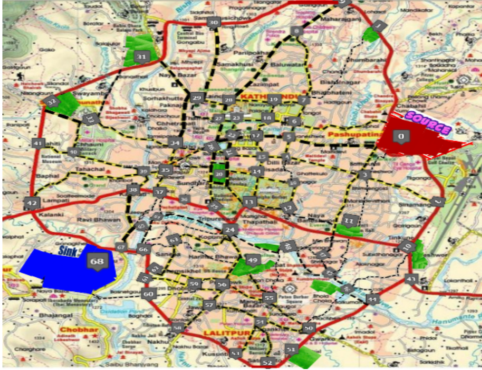
Figure 2.9: Evacuation zone with 69 nodes. Nodes 0 (red) and 68 (blue) represent the source and sink, respectively, whereas green areas are intermediate shelters. (Source: https://www.greattibettour.com/nepal-tours/maps-of-kathmandu.html )
