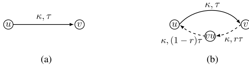
Figure 2.16: Anti-parallel path decomposition (b) of given arc (a) with capacity and transit time.
