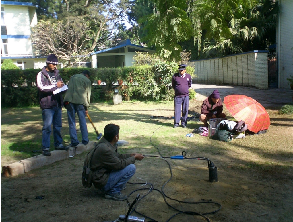
Fig. 4.4: Field layout for P-wave and S-wave data acquisition.
