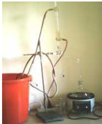
C. Clevenger's oil extracting apparatus.
