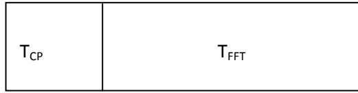
Figure 8: Total duration of an OFDM symbol
