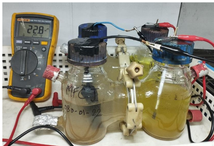
Figure 5 Dual chambered MFC operated with Bagmati River water at 28°C
