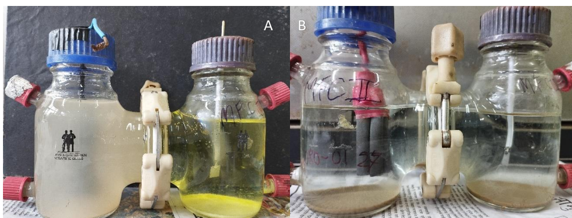
Figure 37 Analyte and Catholyte after MFC Operation of 8 days (A: Synthetic water, B: Bagmati water)
