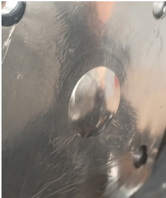
Figure 4.12: Formation of convex surface of diaphragm before reaching burst pressure ratio
