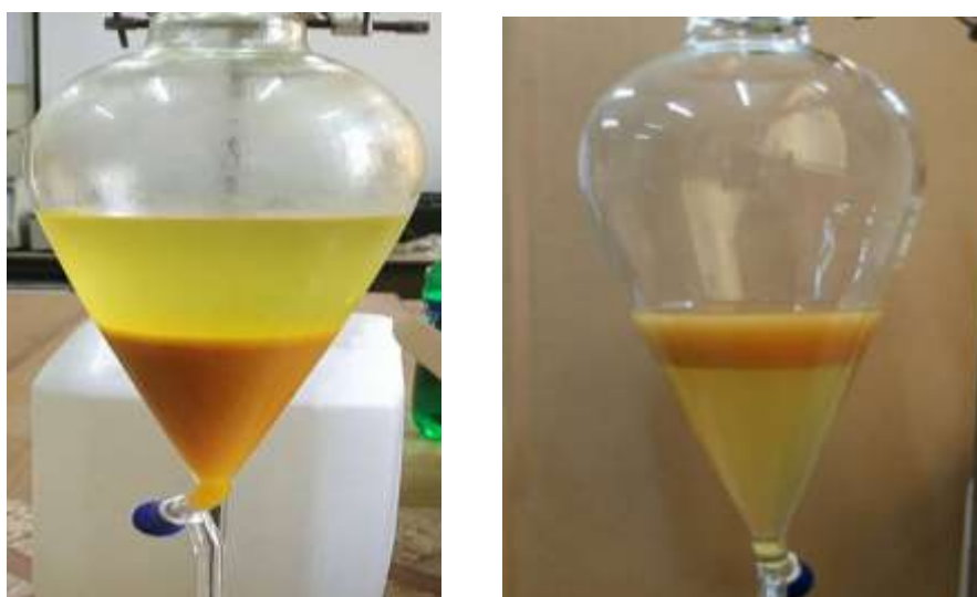
Figure.5. Solvent- solvent partitioning by Hexane and DCM.
