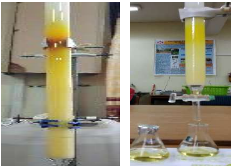
Figure 7. Sephadex gel filtration of DCM fraction
