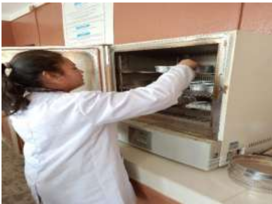
Photo 3: Determination of moisture in hot air oven distiller
