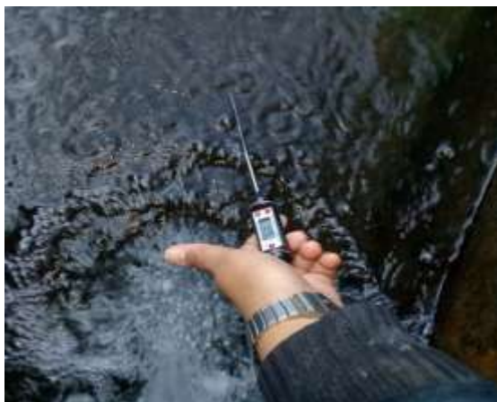
Photo 3: measurement of temperature of raceway using digital thermometer
