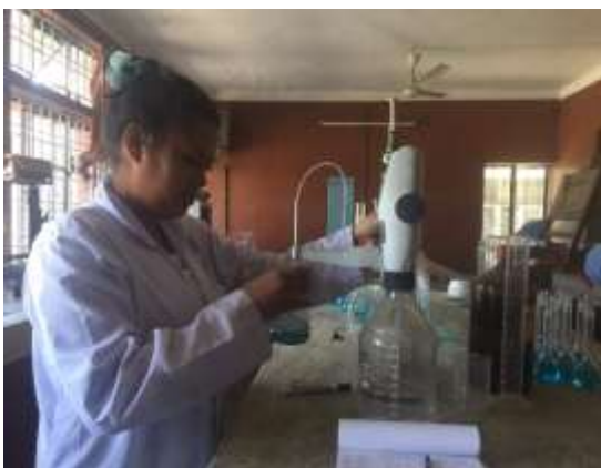
Photo 5: Titration of distillate with 0.03N H_2SO_4 to determine protein
