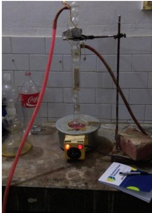
Photograph 1: Extraction Phytochemical by Soxhlet apparatus
