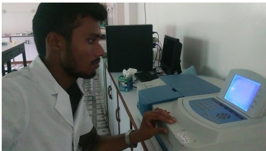
Photograph 4: Measuring antioxidant activity on UV-Visible double beam spectrophotometer in Molecular lab(STC)
