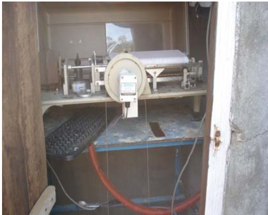
Plate 5: Automatic Gauge recorder on Narayani River at stationno 450, Ferry
