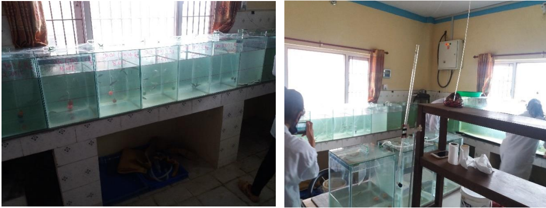
Photo plates 1: Experimental set up for acute toxicity test.
