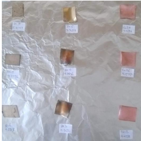
Photograph 2. Short-term colour change in metal sample immersed in fresh pigeon excreta.
