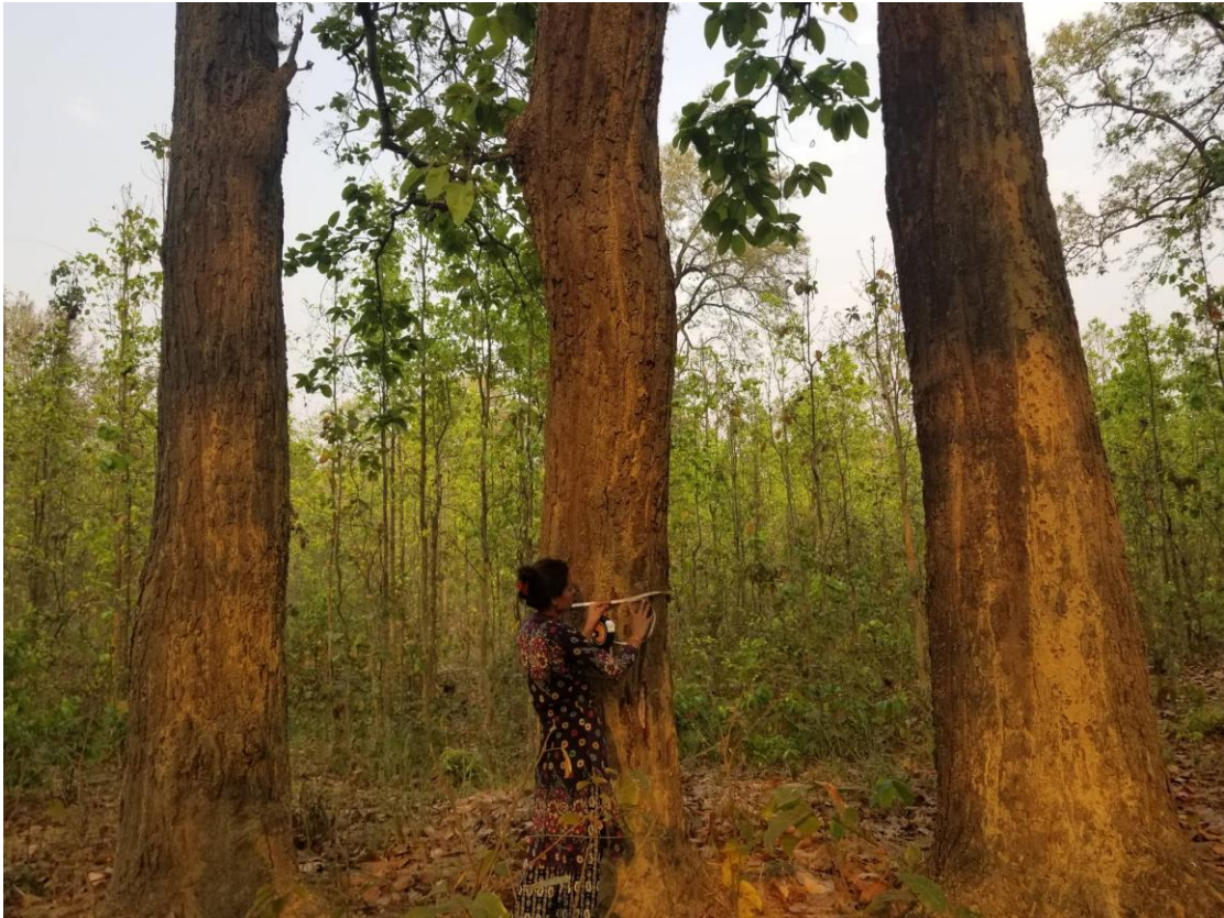
Measuring tree DBH at height 1.37 meter.
