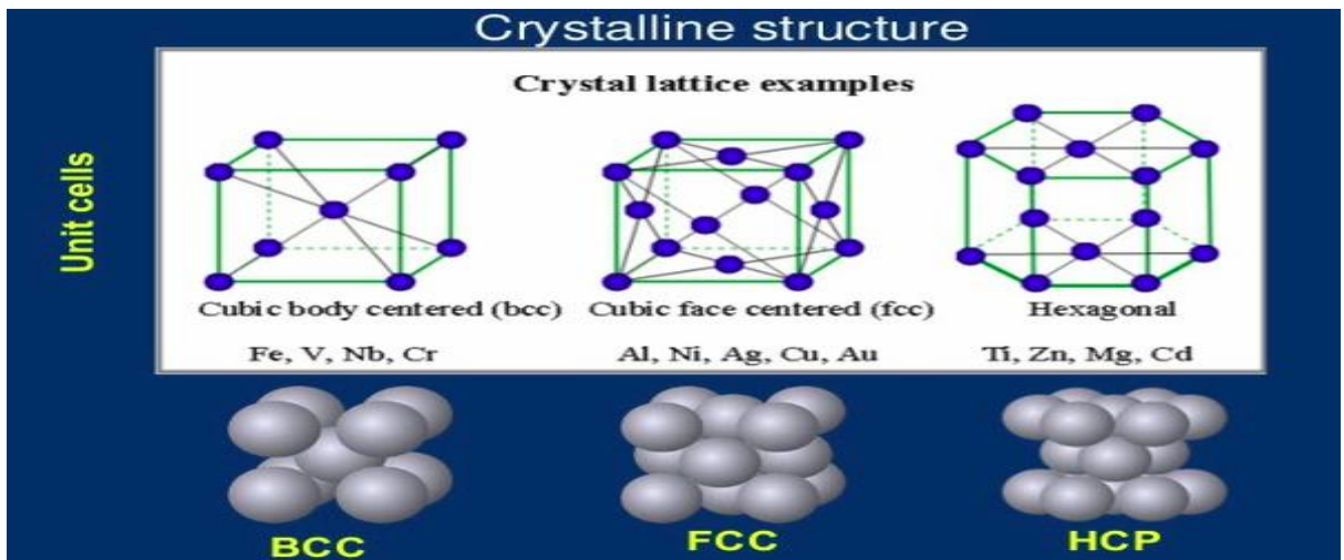
Fig. 1.9: Crystal structure of bcc, fcc and hcp phase [54]
