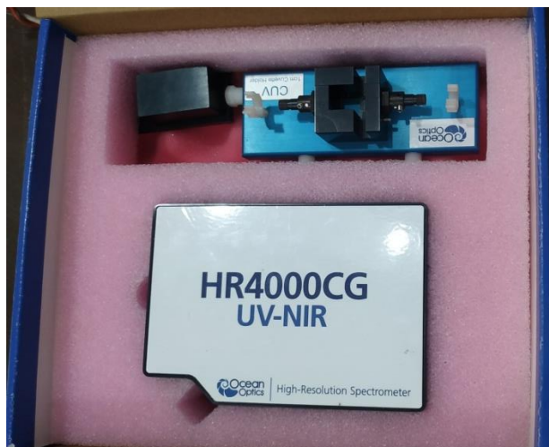
Figure 3.4 UV-Vis spectrophotometer (HR4000CG UV-NIR, Ocean Optics) [At Amrit research lab]
