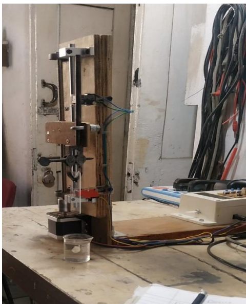
Figure 3.1 Homebuilt Dip Coating Device [At Amrit research lab]
