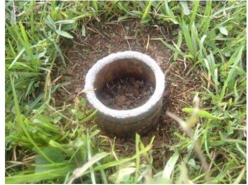
Photo 8: Soil core sampler placed in the plot after removing the above ground vegetation
