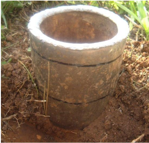
Photo 9: Soil core sampler with markings at 5cm and 10cm height
