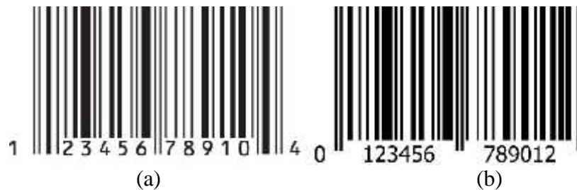
Figure 1.3 (a) Universal Product Code (UPC) - A barcode symbol. (b) European Article Number (EAN) - 13 barcode symbol
