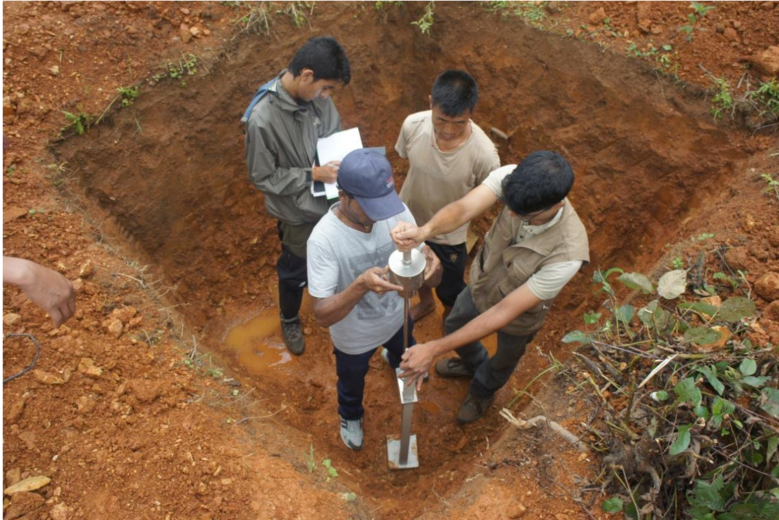
Fig. 3.3: Conducting DCP test in the field.
