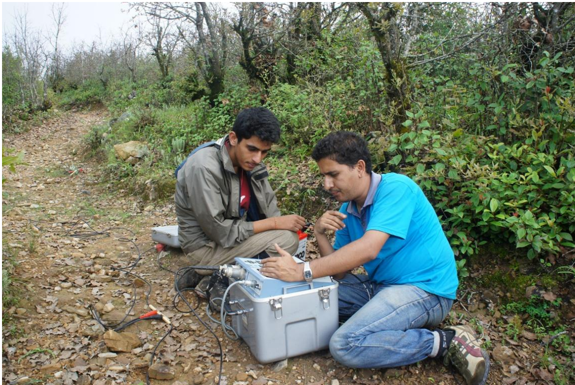
Fig. 3.12: Conducting seismic refraction survey in field.
